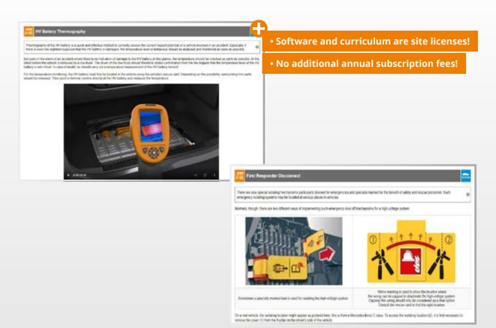
HV battery thermography is a quick and effective method to correctly assess the current hazard potential of a vehicle involved in an accident. Especially if there is even the slightest suspicion that the HV battery is damaged, the temperature level or behaviour should be analysed and monitored as quickly as possible.
