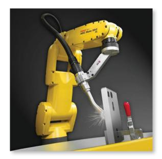
The FANUC ARC Mate 50iD/7L is a high-speed ARC welding robot that is equipped with added reach. Its standard IP67 rating gives it the versatility to work in a variety of different harsh manufacturing environments including dusty and wet areas. With 6 axes, this robot can carry up to 7kg while creating precise arc welds.
